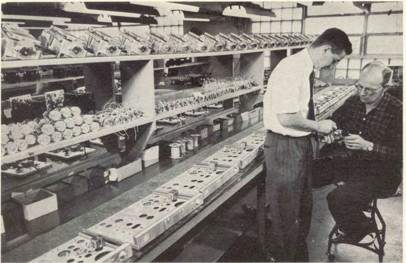
Instrument Is Assembled by skilled craftsmen working from the prototype and detailed drafting prints. A small quantity of instruments is assembled by one man to assure highest quality. Oftentimes, as
