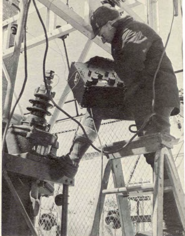
Measuring Leakage Resistance of a large power transformer with a GR Impedance Bridge. Many General Radio instruments are portable and completely self-contained, bringing laboratory accuracy to the field.
