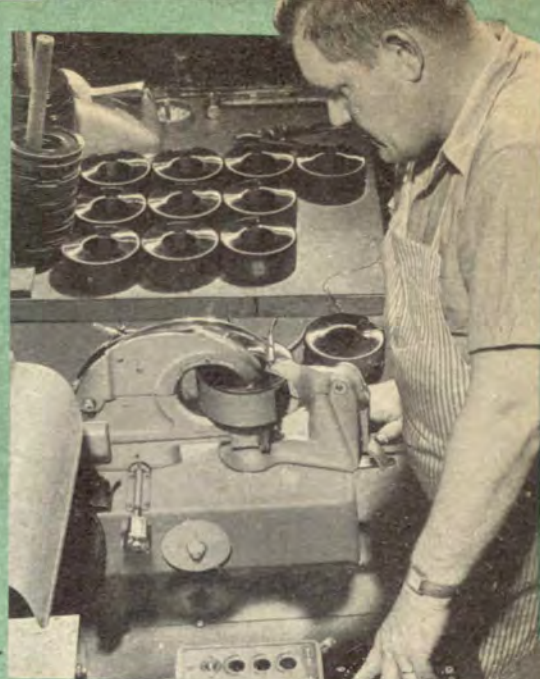
→ Coils For Variac® autotransformers are wound on this unique GR-designed machine, which applies an evenly spaced winding, accurately banked on the inner face, to the toroidally shaped core.
